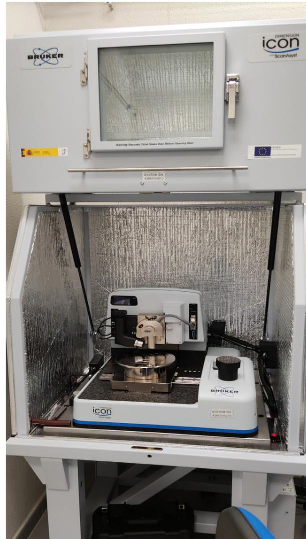
Figura 1. Microscopio AFM Bruker Dimension ICON.
